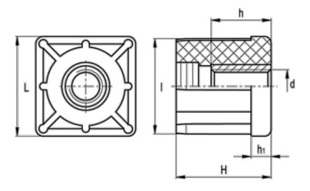
$\begin{array}{lll} d & = M16 \\ h & = 15 \\ H & = 38 \\ h1 & = 8 \\ Internal tube size = 37.0 \\ I & = 37.0 \\ L & = 40 \\ Outer tube size & = 40 \\ \end{array}$
